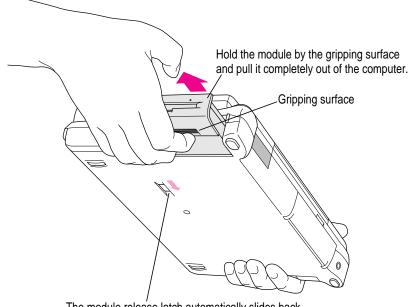
The module release latch automatically slides back into its proper position as you remove the module.
